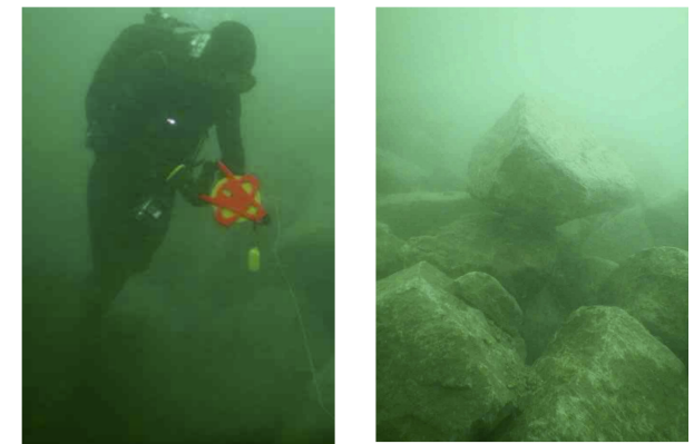
Reef quarry rock with SCUBA diver taking measurements
